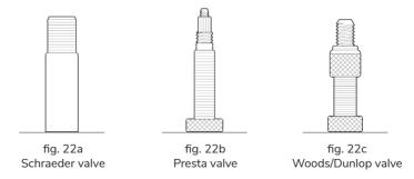
The Presta valve (fig. 22b) has a narrower diameter and is only found on bicycle tires. To inflate a Presta valve tube using a Presta headed bicycle pump, remove the valve cap;
