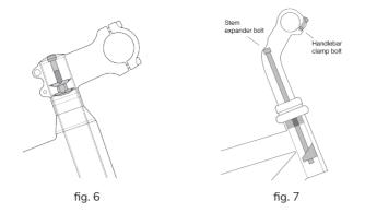
A quill stem has an etched or stamped mark on its shaft which designates the stem's "Minimum Insertion" or "Maximum Extension". This mark must not be visible above the headset.
