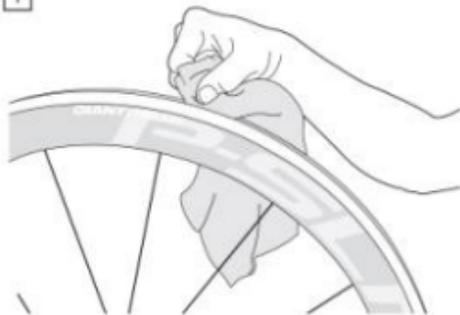
1. Clean and degrease the rim. 50% isopropyl alcohol is recommended.
