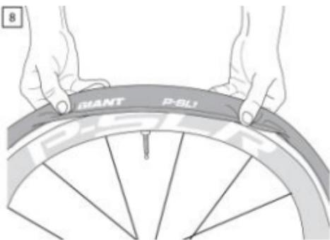
8. Install the tire onto the rim. Make sure the tire beads are seated to the rim evenly before inflating.
