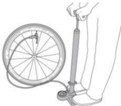
9. Inflate tire to maximum pressure allowed by the rim or tire; make sure the tire fits to the rim properly.
