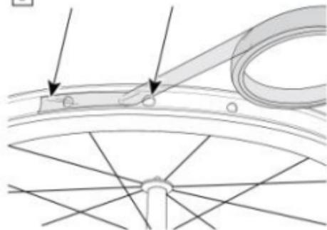
2. Start 3-5 cm left of valve hole and start applying the tubeless conversion tape in a clockwise direction.
