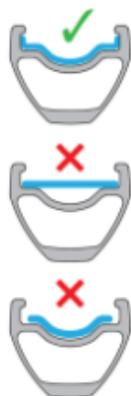
GIANT does not recommend tape width for your specific wheels; different rims with the same ETRTO may require different tape width due to the inner edge dimensions of the rim. Use a tape width that fully covers the surface of the rim bed.
