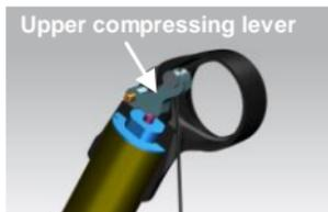
Thread the remote control cable through the hole in the saddle clamp body. Hang the remote control cable stopper on the compressing lever.
