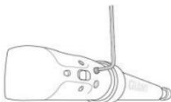
Remove the cartridge fixing screws from saddle clamp body using a 2.5 mm hex key. Pull out the cartridge.
