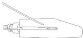
Thread cable to the cable hole.
