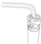
Remove the lower cap using a 8mm hex key.
