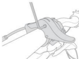
Adjust the cable so the cable casing, barrel and remote unit are tightly connected so the control lever is properly positioned and the cartridge moves properly. Fasten the screw using a 2mm hex key.
