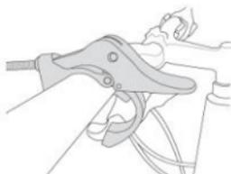
Mount the control unit to the handlebar and fasten with 3mm hex key.
