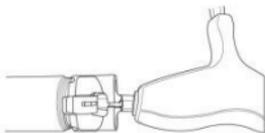
Fasten the lower cap to the recommended torque setting.
