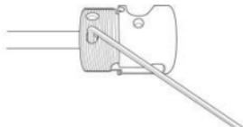
Attach the cartridge to the lower cap. Fasten the cartridge screws to the recommended torque.
