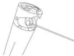
Hang the remote control cable stopper on the lower compressing lever.
