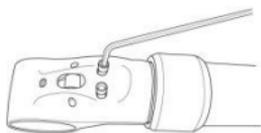
Insert cartridge to the seatpost lower tube to the end. Fasten the fixing screws.
