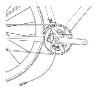
Connect the charging cable to a USB power source. For best results, we recommend using a dedicated USB charger with output current of 1~2A.
