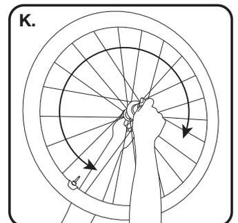
CADEX Tubeless Tires use a coating on the inside of the casing to enhance the tire's air retention properties. As this coating is vulnerable to damage from tire levers, it is recommended to install and remove the tire without using tire levers or by using CADEX's specifically designed tubeless tire lever.
