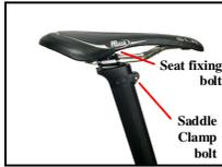
**CAUTION :** Before clamping any item to the seat post, make sure the clamp is free from any burrs or sharp edges. This does not only apply to the Saddle clamping mechanism that holds the saddle, but also the clamps of other accessories, such as tail lights, reflectors and bags that might be fixed to the seat post.
